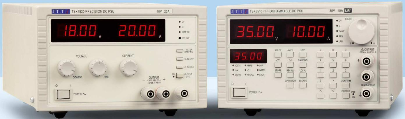
350/360 watts, standard and bus programmable
